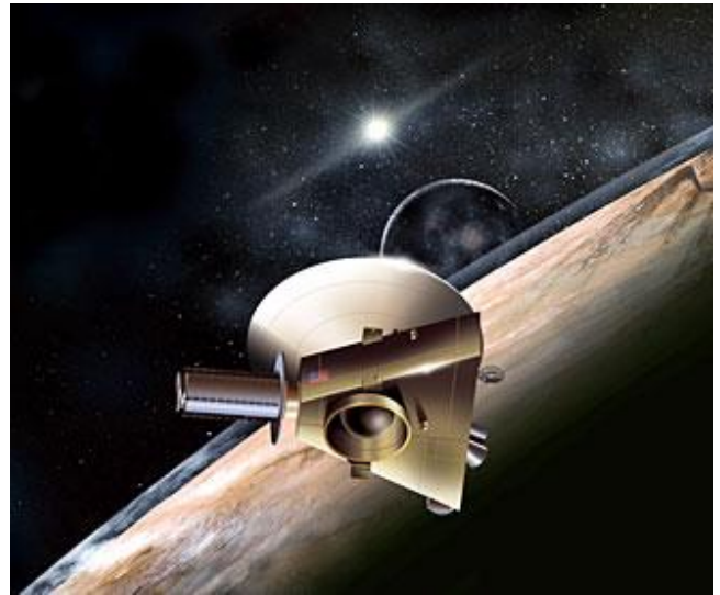
An artist's concept of the New Horizons spacecraft. The craft's miniature cameras, radio science experiment, ultraviolet and infrared spectrometers and space plasma experiments will characterize the global geology and geomorphology of Pluto and Charon, map their surface compositions and temperatures, and examine Pluto's atmosphere in detail. The spacecraft's most prominent design feature is an 8-foot dish antenna, through which it will communicate with Earth from as far as 4.7 billion miles away. Photo: Johns Hopkins University Applied Physics Laboratory/Southwest Research Institute (JHUAPL/SwRI)
